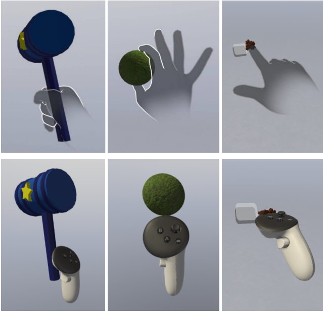
Figure 3: Interactable objects. The first row shows the objects for the hand tracking conditions: a hammer (grasp), a seed (pinch), and a button (tap). The second row shows the corresponding objects in the controller conditions.
